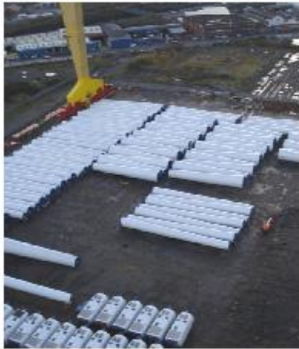
Port storage for towers and nacelles
