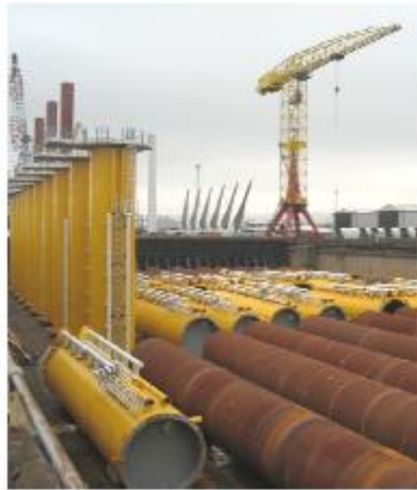
Port storage for monopiles
